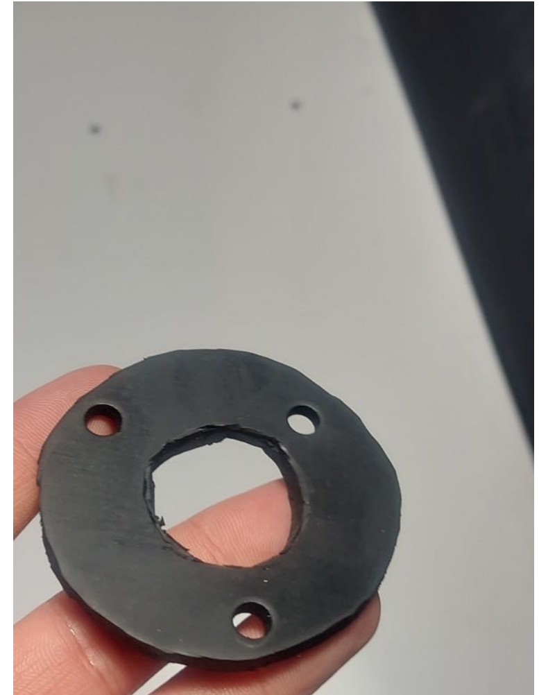
A neoprene rubber gasket cut for the open source MFC
